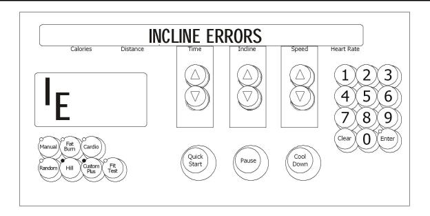
Upon entry into this test the letters IE (incline errors) will be in the profile window. This test allows seeing the current lift motor error conditions. The following is a list of the current lift motor error conditions. If an error is displayed, refer to the troubleshooting section for corrective action.
